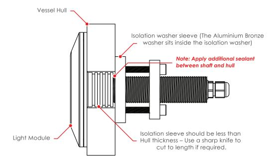
Note: A suitable marine adhesive (e.g. 3M - 4200) should be used between the light module and the isolation sleeve and the isolation sleeve and the hull of the vessel. This diagram shows the order of assembly. It may look slightly different from product to product, but the assembly order is the same.
