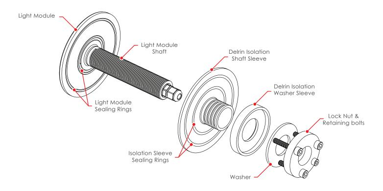
How to assemble the isolation shaft and washer sleeve
