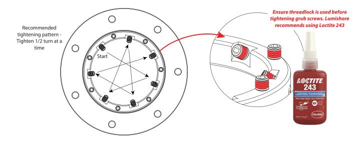
6) USING A SUITABLE TORQUE DRIVER SET TO **3 Nm**, tighten the VERTICAL grub screws one turn at a time, working in a cross tightening pattern (i.e. move to a screw opposite the one you have just tightened - DO NOT move to the next screw in the circle - see diagram below). Tighten until each screw achieves the desired torque.
