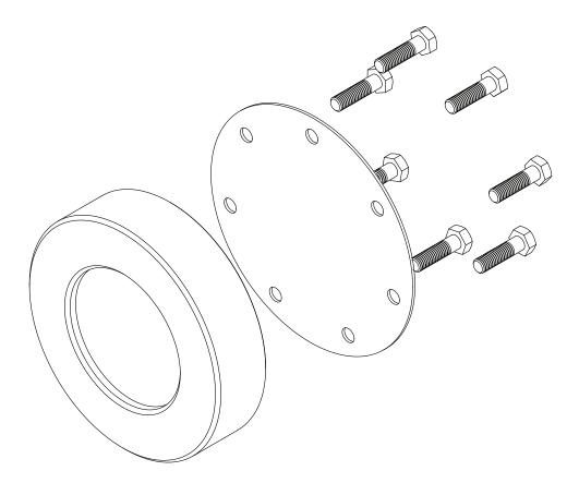
NOTE: Keep the rear cover plate fitted until it is time to install the lens and light module.
