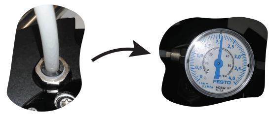
5) Close the valve, and monitor the pressure for 30 seconds. Check that there is NO DROP IN PRESSURE.
