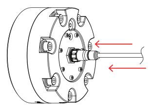
NOTE: The cable can be fitted at any time. If the cable is not fitted at this stage ensure that the DUST CAP IS IN PLACE on the back of the light.
