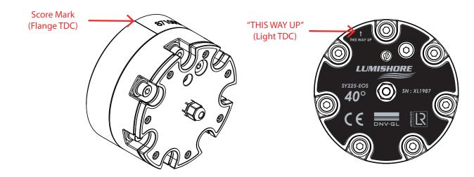
6) Tighten the bolts in a criss-cross pattern (as shown in the diagram). Tighten the bolts half a turn at a time, then move on to the next bolt. USING A TORQUE WRENCH tighten the bolts to a torque of 15 Nm.
