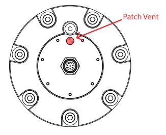
8) Ensure there is no debris or water in either connector. Fit the cable to the back of the light (SY220 and SY250). Ensure that the key on the cable connector, and the key on the light connector line up. Screw the connector home. The connector should fit easily - DO NOT force the connector.
