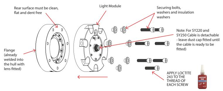
5) Apply a small amount of Loctite 243 (supplied) to the thread of each bolt before fitting. Fit the light module to the flange, and secure in place using the bolts - MAKE SURE that the bolts have the washer and nylon insulating washers fitted.
