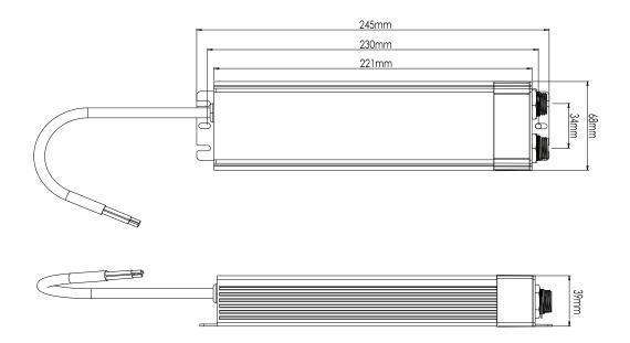
Input Voltage Range: 90-240VAC (50/60Hz)
