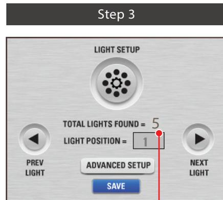
The controller will detect how many lights are connected and then display the result on the screen. Check if the number of lights matches the number of installed lights, if not please refer to the troubleshooting guide at the back.
