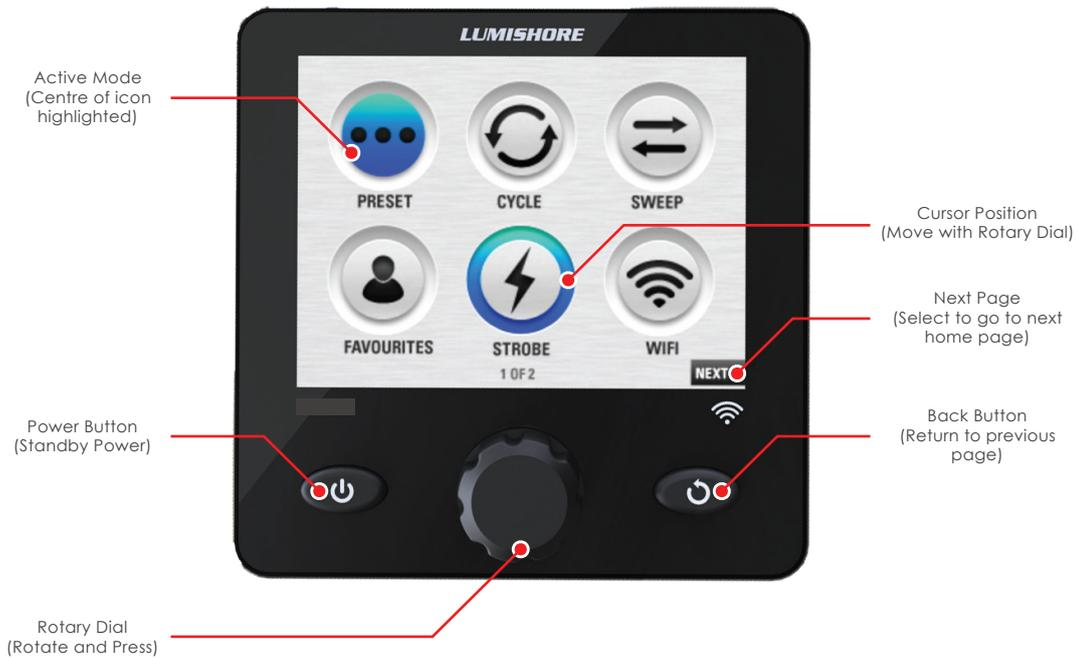
The EOS control interface is very easy to use, use the rotary dial to move the cursor around the screen, pressing the rotary dial will select the icon/slider bar or text that is highlighted. The icon will change color to show it has been selected.
