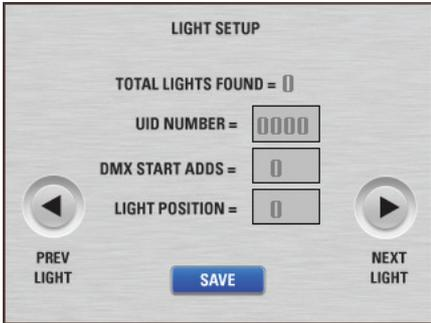
UID (unique Identification number): This number is an identification code that is unique to every Driver. The code cannot be changed and is for reference only.
