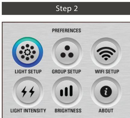
Select Light Setup Mode. If this is a new setup, the Controller will then enter "Discovery" mode where it searches for connected lights. To "Add" lights or "Modify" an existing setup - see next section.
