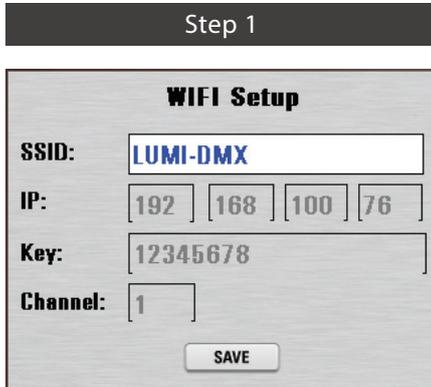
Make a note of the SSID name and password KEY in the Wi-Fi setup Mode in setup.
