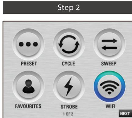
Once the information has been recorded return to home page and select Wi-Fi mode. The internal Wi-Fi will be activated. Note: exiting this mode will turn the Wi-Fi off again and the controller will not be found by the iPhone.
