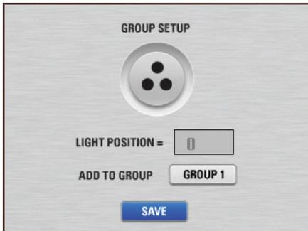
The position of lights can be placed into groups for easier reference and control within "Scenes" mode.
