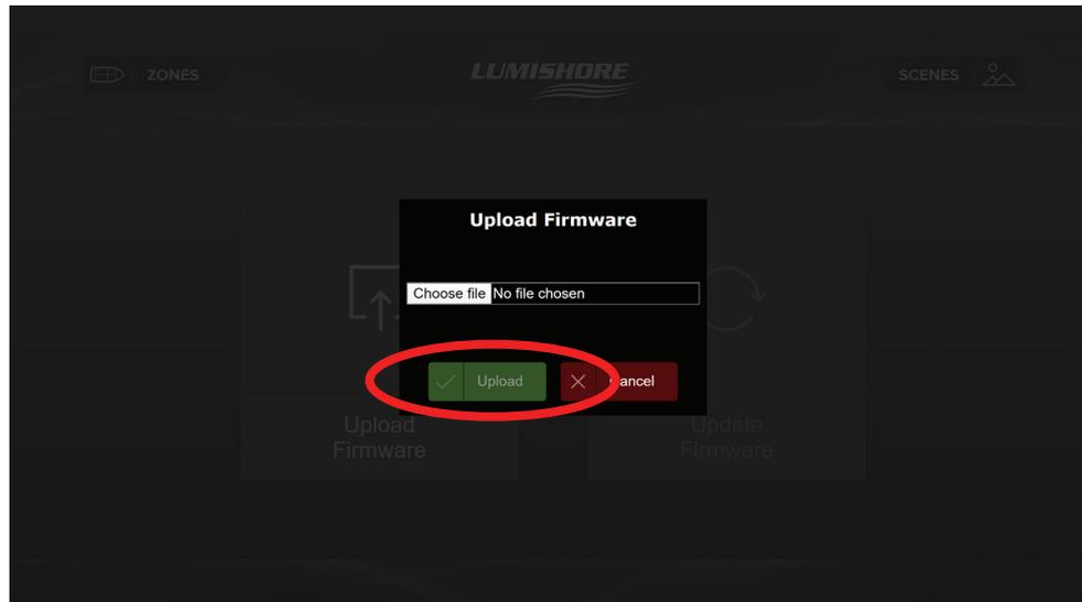
Once the file has uploaded you can choose to install now or install at a later time. Select install now to complete the firmware update. (the process can take 30-50 minutes), please ensure the PC or laptop and Lumi-Link Command Center are left uninterrupted during this time.
