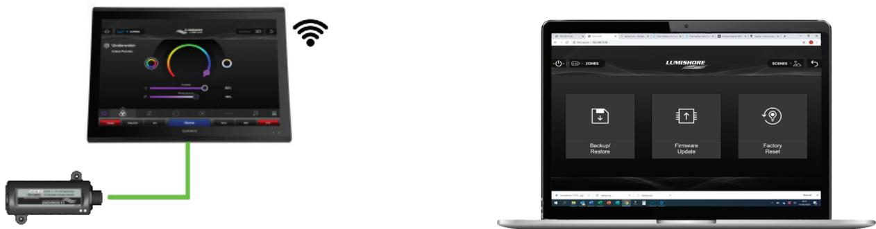
Using the connected device navigate to the “System Maintenance” menu and select “Firmware Update”
