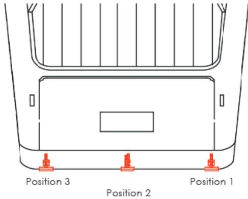
The position of the lights around the vessel can also be setup. This ensures that sweep mode works in the correct order.
