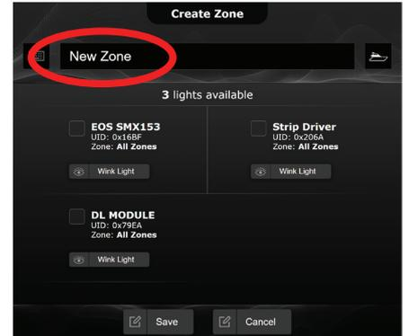
Use the name of the light or "Wink Light" to identify each light on the network. Select which lights to allocate to the zone and then save the selection.
