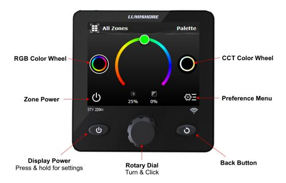
The EOS-LUX SUPRA Display is very easy to use, It is a touch screen device but can also be used with the rotary dial. Use the rotary dial to move the cursor around the screen, pressing the rotary dial will select the icon/slider bar or text that is highlighted.
