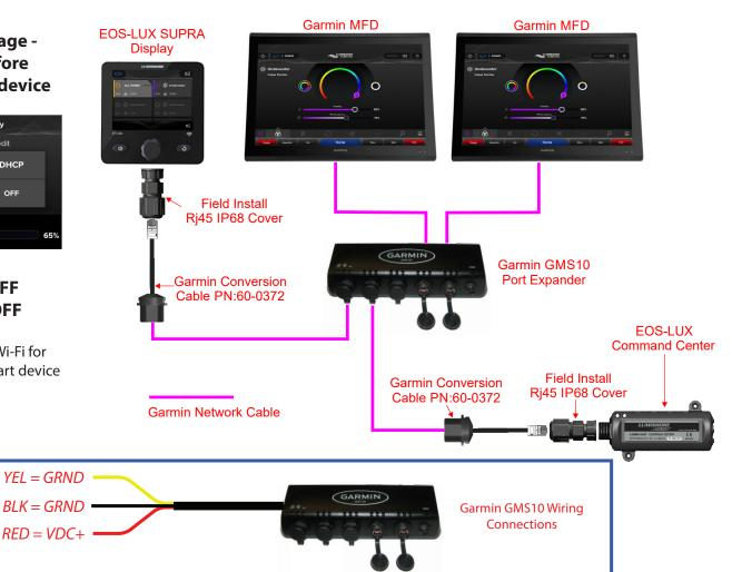
Note: To prevent the GMS10 switching off when the MFD is turned off connect its yellow wire to Ground.
