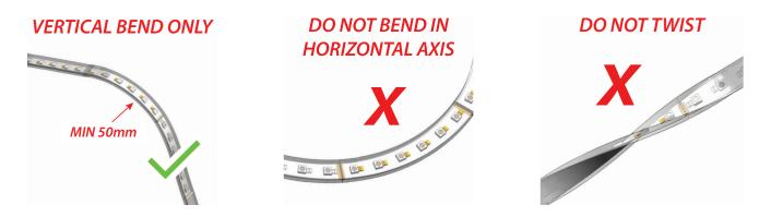
**DO NOT** allow the strip light to drop or twist during install - uncoil it carefully from the reel **DO NOT** apply pressure to the strip in the area of the LEDs - press the edge of the strip only **DO NOT** pull, stretch, twist or bend the strip in the horizontal axis
