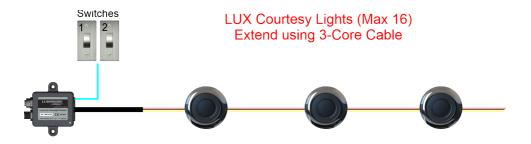
NOTE: The Lumishore Lux Courtesy Light CL25 requires connection to the Lumishore Lux Light Module. For full electrical installation and wiring diagrams please refer to the Lux Light Module installation guide.
