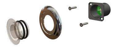
**CLEAR** marine sealant should be used between lens and bezel and behind the bezel (see below), ensure no sealant contacts O-rings. Fit lens and O-rings through the bezel and clean any excess adhesive using a soft cloth and soap and water - **DO NOT USE CHEMICAL CLEANERS**.
