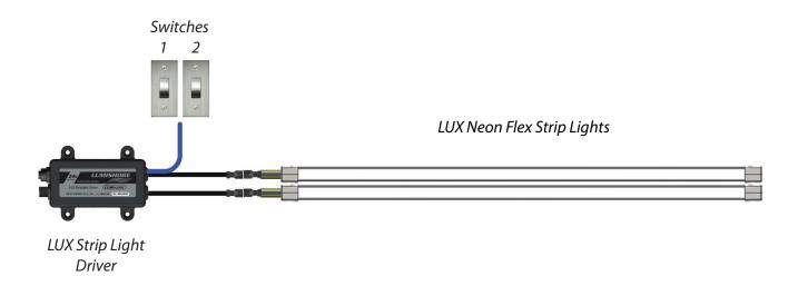
NOTE: The Lumishore LUX Neon Flex Strip Lights requires connection to the Lumishore LUX Strip Light Driver Module. For full electrical installation and wiring diagrams please refer to the LUX Strip Light Driver Installation Manual (45-0143).
