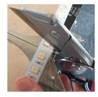
3. Using a pair of scissors cut the strip light to length. Use a single cutting motion in the center of the cut pads.
