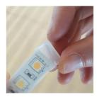
Fit end cap, clean up any excess adhesive. Allow to cure for 24hrs before handling.
