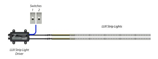
NOTE: The Lumishore Lux Strip Lights requires connection to the Lumishore LUX Strip Light Driver Module. For full electrical installation and wiring diagrams please refer to the LUX Strip Light Driver Installation Manual (45-0143).
