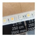
Locate the closest cut point to the length required.
