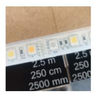
1. Locate the closest cut point to the length required.
