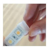
6. Fit end cap, clean up any excess adhesive. Allow to cure for 24hrs before handling.
