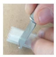
1. At the end to be sealed, peel back 20mm of the adhesive backing and very lightly score the adhesive 10mm from the end using a sharp blade.
