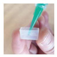
5. Half fill the end cap with silicone adhesive (supplied)
