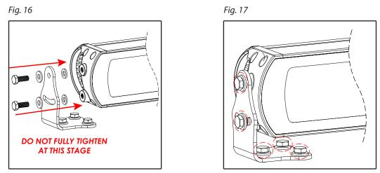
8. Return the light to the marked angle (fig. 18). Bolts on the sides of each bracket can now be tightened to a final torque of <u>8Nm</u>. Only once the light has been angled and side bolts tightened can the brackets be tightned down.
