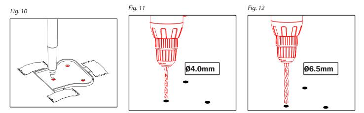
6. Remove brackets from light. Using the supplied fixing hardware fix the brackets to the boat. It is recommended that marine sealant (3M 4200) is used in and around the mounting holes. The spreader plate is required to go underneath the mounting surface and provides an even distribution of force when tightening. It is important to note that at this stage these mounting bolts are to be left loose as this is a crucial step in adjusting the angle of the light in the coming steps.
