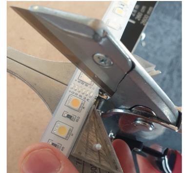
1. Locate the closest cut point to the length required.
