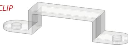
Using suitable screws the fasteners should be placed every 250 - 300mm (9.842 - 11.811 in) apart and/or at either side of the bend. For best results do not position in line with LED's.
