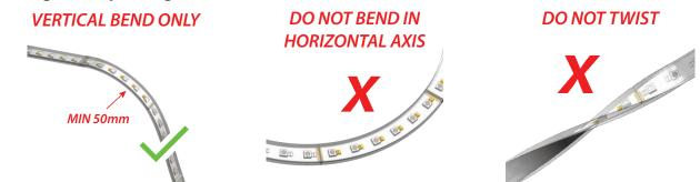
**DO NOT** allow the strip light to drop or twist during install - uncoil it carefully from the reel **DO NOT** apply pressure to the strip in the area of the LEDs - press the edge of the strip only **DO NOT** pull, stretch, twist or bend the strip in the horizontal axis
