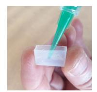
5. Half fill the end cap with silicone adhesive (supplied)
