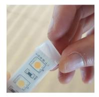
6. Fit end cap, clean up any excess adhesive. Allow to cure for 24hrs before handling. Do not use chemical cleaners
