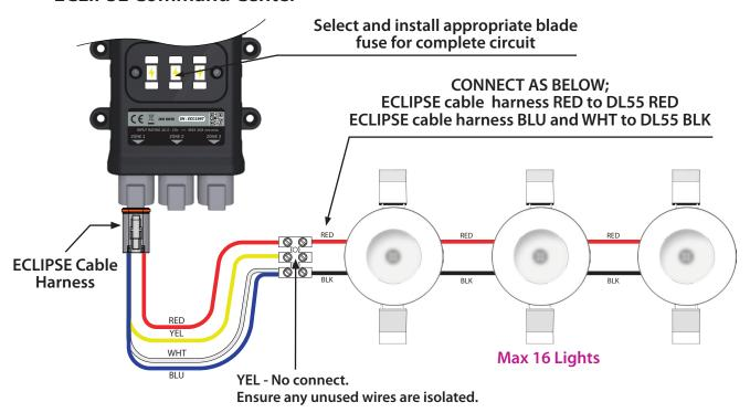
Note: Single color and dual color lights should not be added to the same zone output. Use a separate zone output for each type
