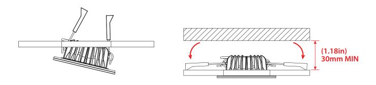
For exterior installations or wet areas it is recommended that the light is fixed in place using a suitable marine sealant / adhesive. *Remove the spring clips and the black gasket* from the fixture and dispense a small amount of adhesive around the glass bezel. Push into place using a slight rotation of the light to spread the adhesive evenly. Clean any excess adhesive using a soft cloth and soap and water – *DO NOT USE CHEMICAL CLEANERS*.
