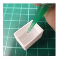
10. Fill the cable exit end cap 1/3 of the way up with silicone adhesive (supplied).
