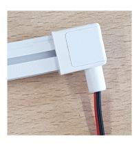
11. Fit end cap over extrusion and push until it stops. Excess adhesive should be wiped away using water ONLY. Use a paper towel to dry and allow to cure undisturbed for 24hrs.
