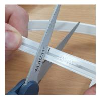
3. Using a pair of scissors cut the Neon Flex to length. Use a single cutting motion in the center of the cut point.
