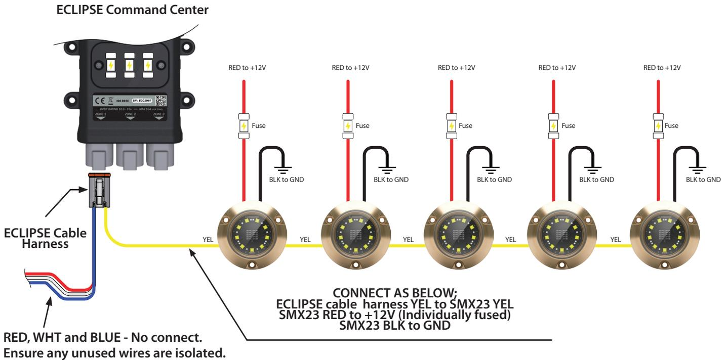
*Note : Single color and dual color lights should not be added to the same zone output. Use a separate zone output for each type.*
