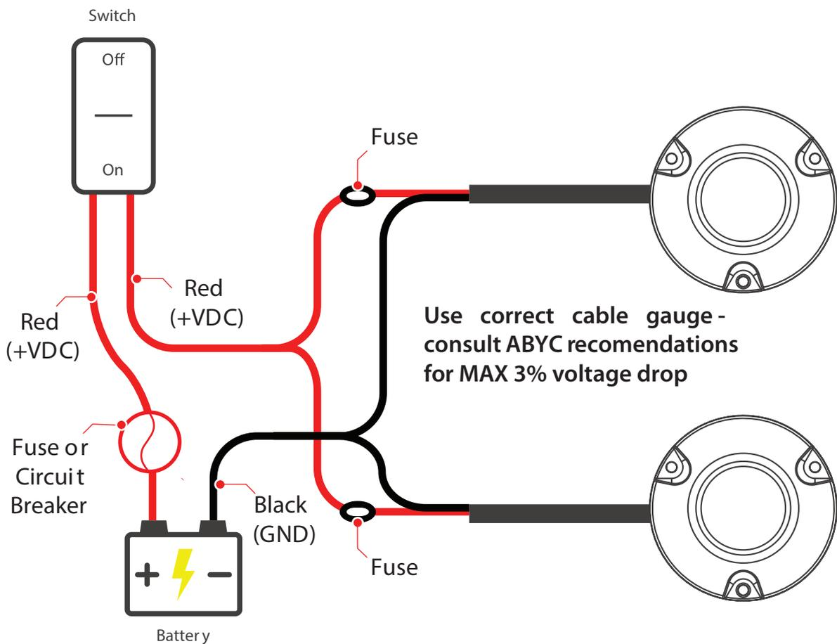
The light cables can be extended. Ensure the correct cable gauge is used to avoid issues with voltage drop. Follow ABYC recommendations for no more than 3% voltage drop. Consult a qualified electrical installer, or contact Lumishore for further information.
