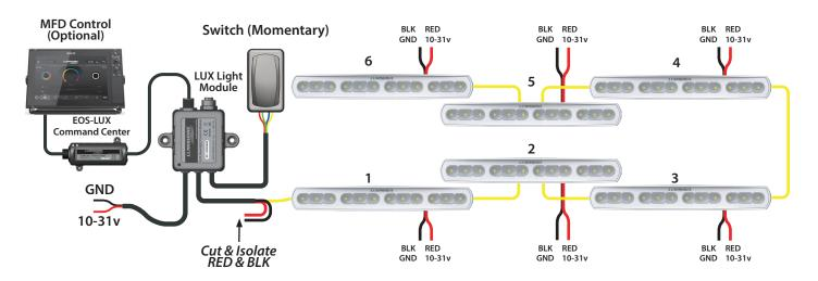
Note: Black wire from each light and LUX Module should connect to common ground
