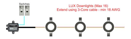
NOTE: The Lumishore Lux downlight DL50 requires connection to the Lumishore Lux Downlight Module. For full electrical installation and wiring diagrams please refer to the Lux Downlight Module installation guide.
