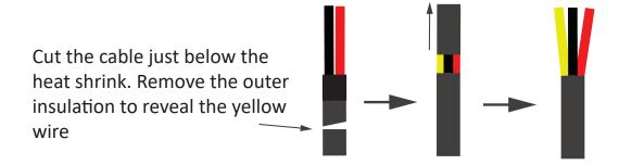
Trim back the insulation on each core to reveal 4mm of wire.
