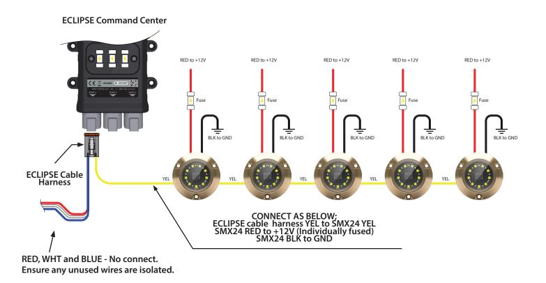
Note : Single color and dual color lights should not be added to the same zone output. Use a separate zone output for each type.
