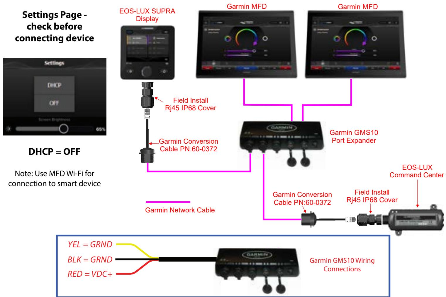
*Note: To prevent the GMS10 switching off when the MFD is turned off connect its yellow wire to Ground.*
