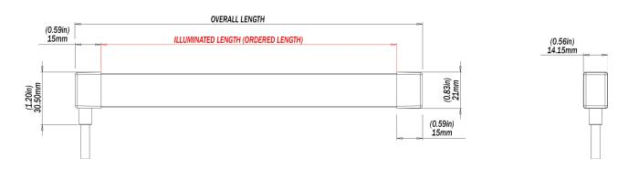
Note - tolerance on illuminated length is +/-  $5\,\text{mm}$
